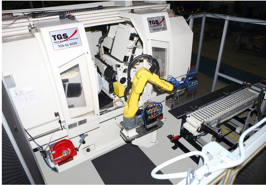
TGS-CL-6020 CNC centerless grinder shown with robot loading/unloading system.
